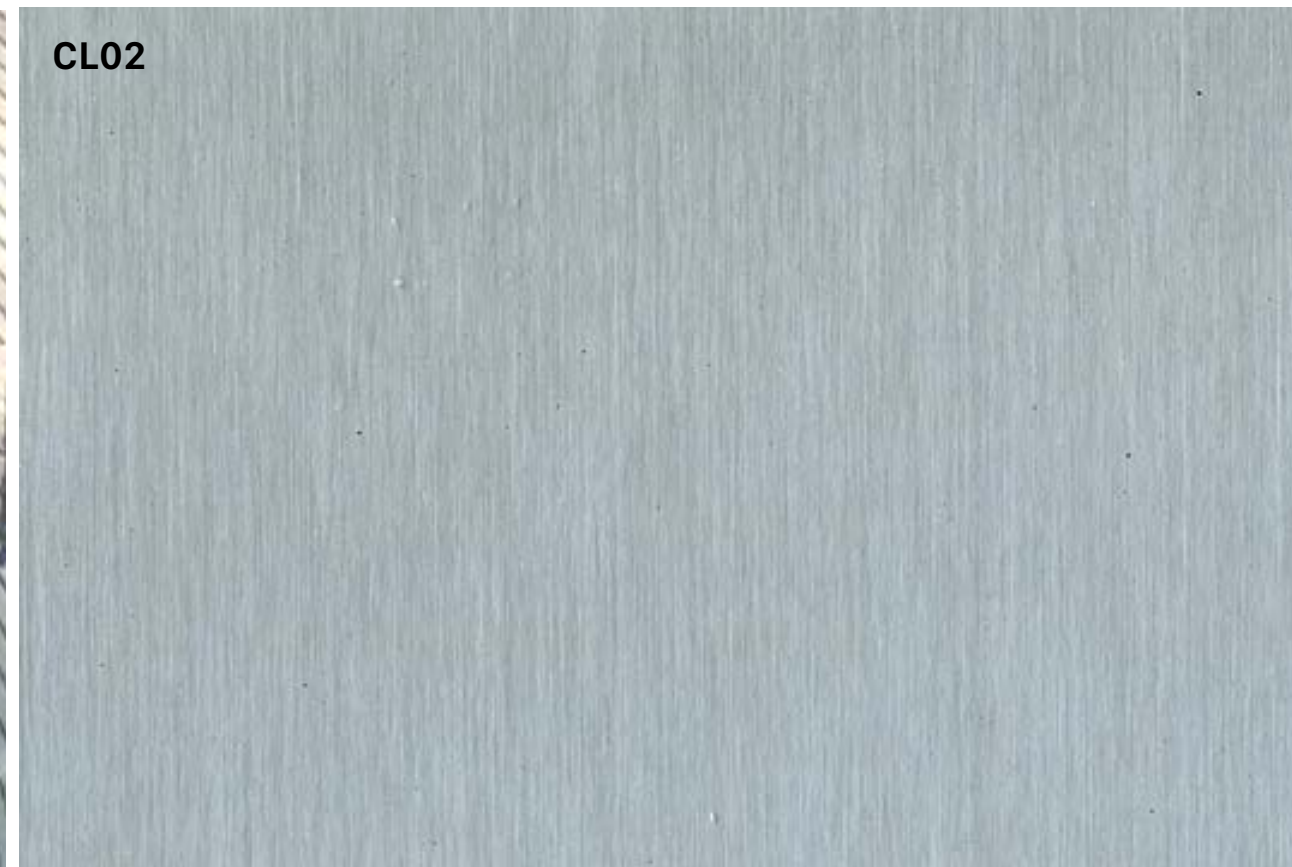
/Material selection: Natural Zinc with pre-oxidised finish (Supplied by VMZinc or equivalent)
